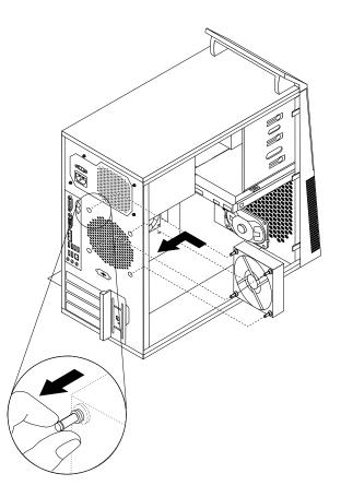
Figure 44. Installing the rear fan
